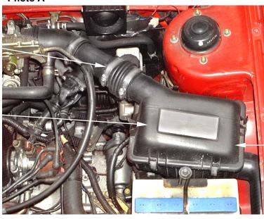
3. Remove the air box base from the inner wing by removing the 3 securing screws located inside of the air box base.
